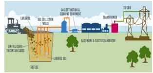
Figure. 1. Landfill Gas Plant Scheme (US EPA, 2010)
