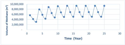
Figure 2. Sustainable Landfill Gas Methane Production Model
