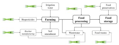
Figure 2. Partial scheme of the possible contributions of hydrodynamic cavitation processes to conventional food production chains. Numbers refer to HC processes applicable to different steps of the food production chains.
