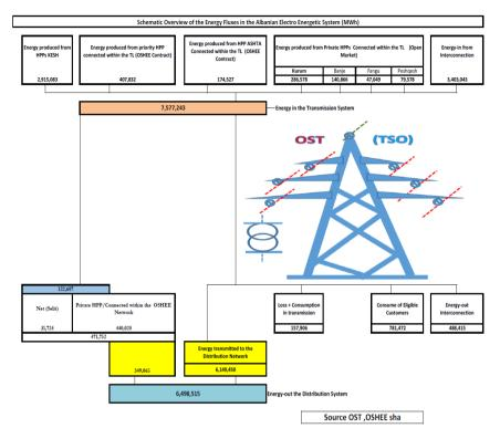
Figure 1. Schematic overview of the Energy fluxes in the Albanian Electro Energetic System. Source: <u>mmw.kesb.al</u>
