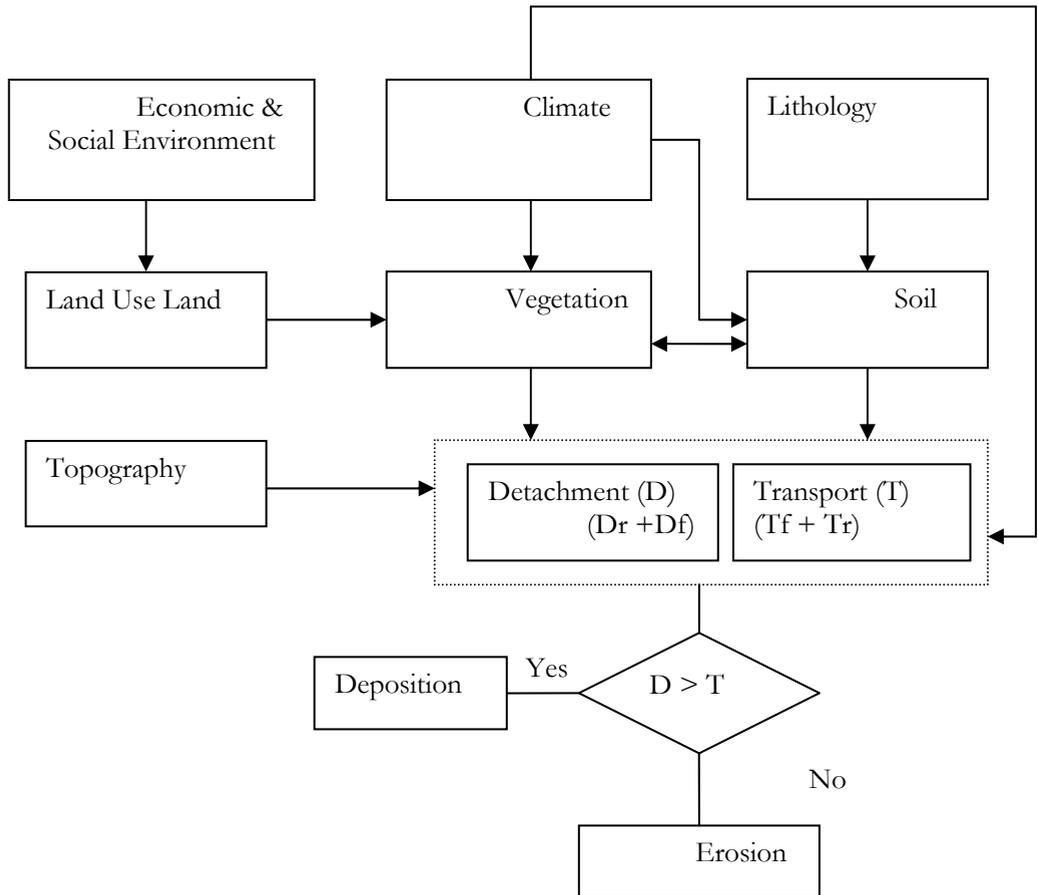
**Figure 1.** Soil erosion process and controlling factors: ( $D_r$  = soil detachment due to raindrop impact,  $D_f$  = soil detachment due to surface runoff or overland flow,  $T_r$  = soil material transport due to raindrop impact;  $T_f$  = soil material transport due to surface runoff or overland flow).
