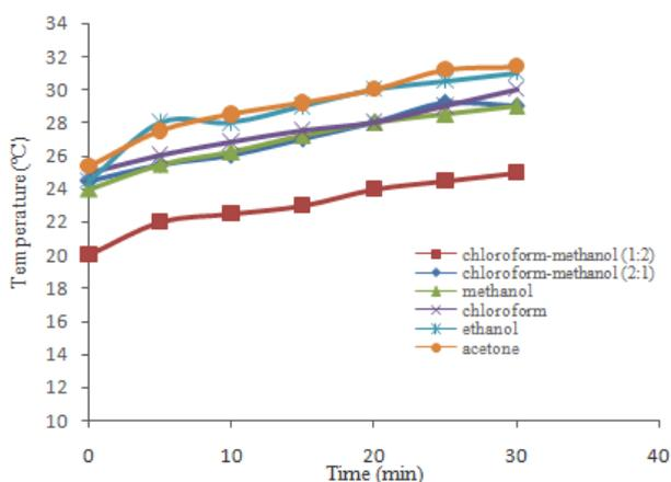
**Figure 5.** Temperature curve of ultrasound-assisted extraction process.
