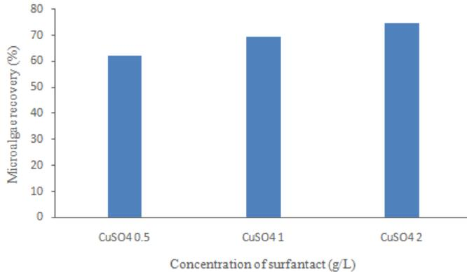
Figure 2. Microalgae recovery (%) for different doses of copper (II) sulphate.
